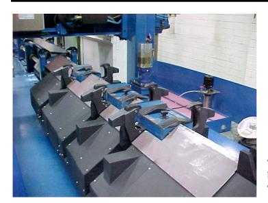
The ACUCUT 12000 is a machine custom built to process truck chassis rails. The machine features include:
